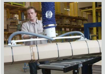
Soft or even deformed cartons are no problem for the Jumbo.
