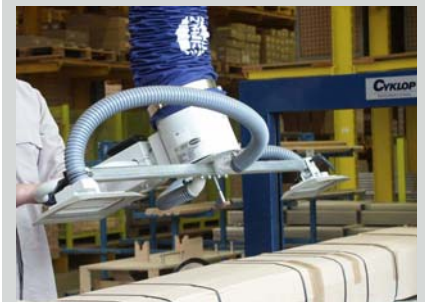
The two suction pads can be adjusted longitudinally for safe handling of cartons of all sizes.
