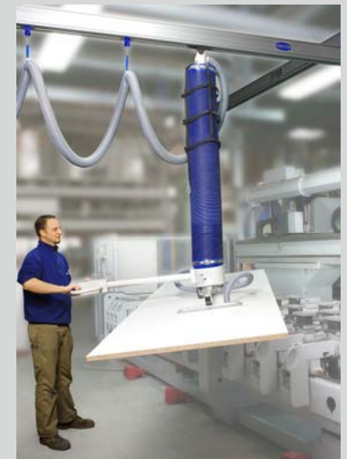
The JumboErgo vacuum tube lifter being used to load a CNC machining centre with chipboards
