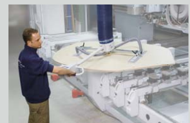
Removing a processed wooden board from the machine table using the vacuum tube lifter JumboErgo
